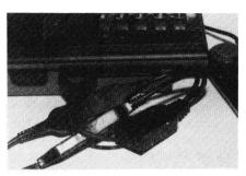
The Altai joystick interface is fully compatible with the PASE standard interface, and works with any Oric computer. It takes one or two Atari compatible joysticks and plugs into the printer port, so may affect the sound of some games.
